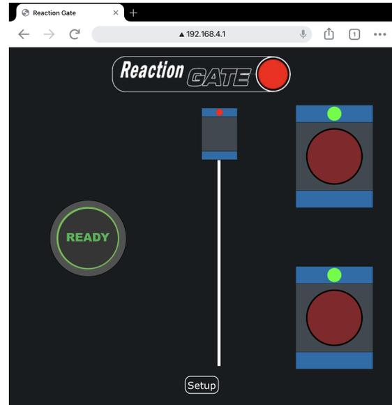
A successful trigger of the Gate at a speed at or above that set in <SETUP>, one of the Light Units will illuminate and this will also be shown in the display. Additionally, an actual speed rating will be shown on the <Ready> button.
