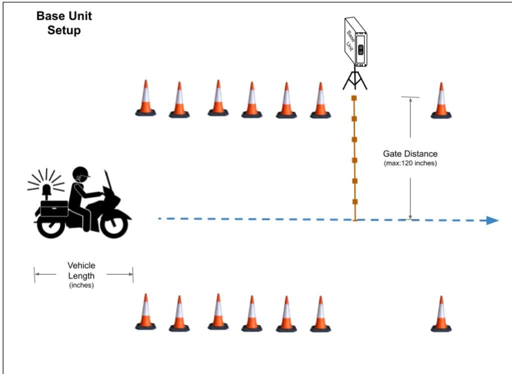
The *Base Unit* must be set up with the *Gate* (beam) pointed across the lane of traffic. A vehicle can be detected up to 10 ft from the *Base Unit* and this parameter is also configurable in **Setup**. Also shown in the above graphic is the Vehicle Length parameter which is utilized in determination of vehicle speed through the *Gate*.
