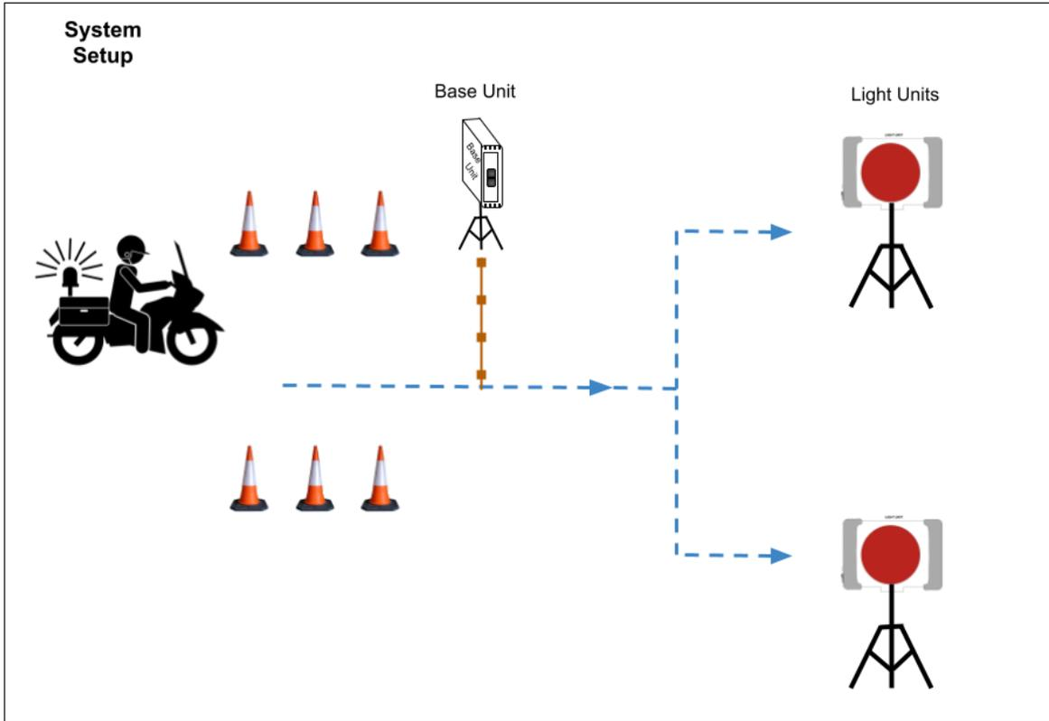
While there can be a variety of applications, the most standard configuration of the **ReactionGate™** is illustrated above with the *Base Unit* as the trigger for randomly illuminating one of the *Light Units*.
