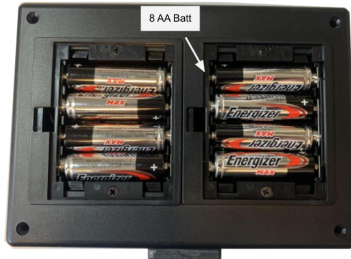
Each Light Unit and the Base Unit has two access doors at the back for replacement of the AA batteries. Install eight new AA batteries (do not mix old and new batteries or various battery types) while paying attention to the polarity indicators.
