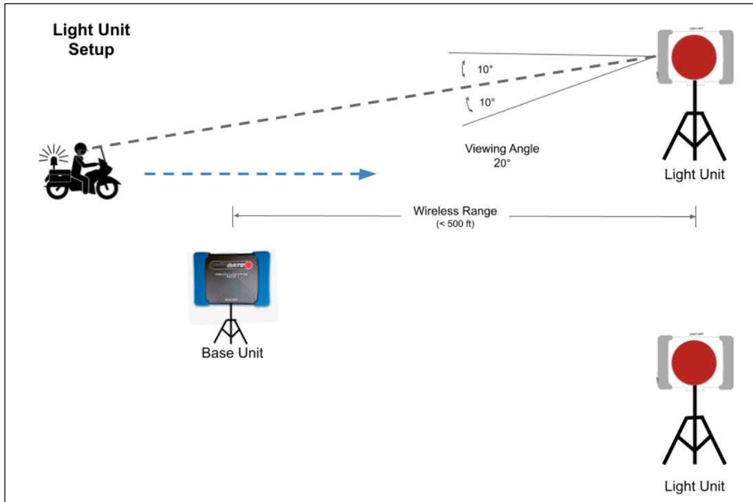
*Light Units* are placed on the course, typically as an indication of an object to avoid. The lights utilized in the system are brake lights and thus have a viewing angle of +/- 10°. While the *Light Units* are typically set up closer to the *Base Unit*, the wireless range between the *Base Unit* and *Light Units* must not exceed 500'. At this distance the *Light Units* may become difficult to see as well.
